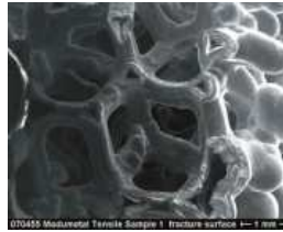
©2008 Modumetal. Ferrous Sample 1. Fracture surface. 100x
